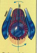
The stepper motor has many (sometimes hundreds) of coils. Switching current from one coil to another causes the whole to rotate in precisely controllable increments of arc
